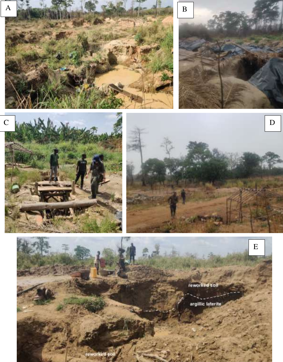
Figure 6-8 - Artisanal miners' activity in the project area at March 2023. A: washing and excavation facility, soil and saprolite. B and C: shafts and trenches to mine quartz veins (depth of 15-20 m); D: former central area of the mining camp, former market. E: washing with a mechanised tool. Note the thickness of reworked soil.
