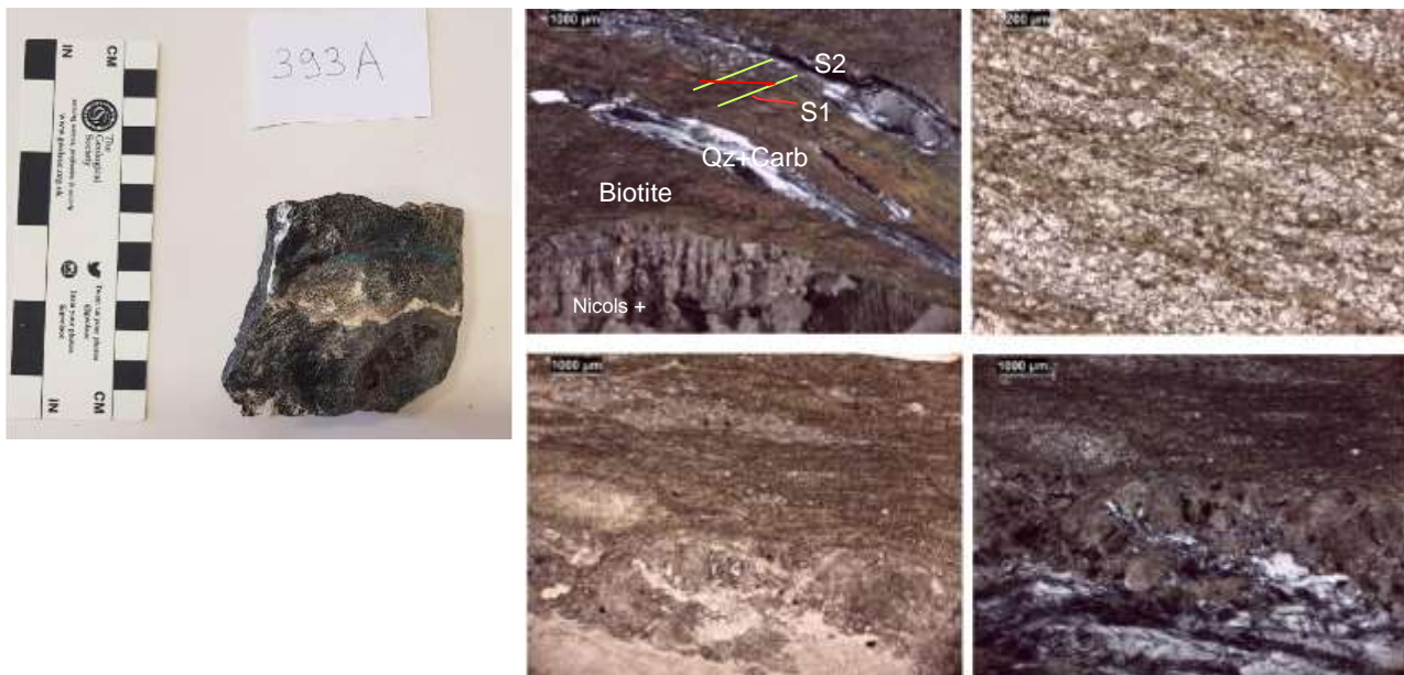
Figure 9-13 - Thin section of the sample 393A observed at optical microscope.
