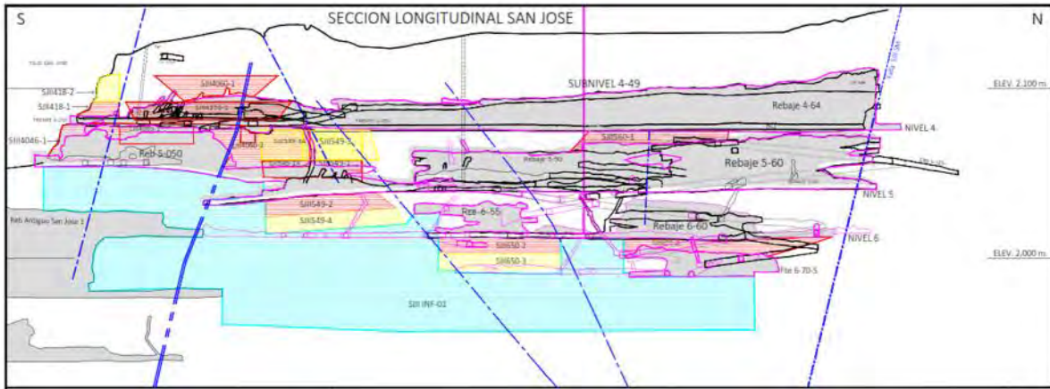
Figure 15- 1: Typical vertical longitudinal section (VLP) showing the blocks of proven and probable ore in the San José II orebody
